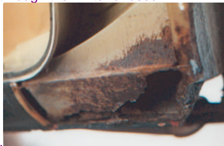
Quarter rear wing cut away to reveal the hidden rear sill corrosion on an MGB
